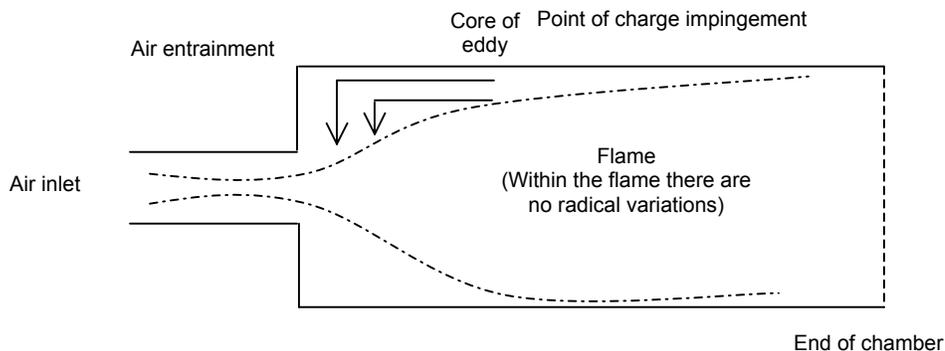
Fig. 2: Combustion Chamber with assumed flow pattern.
