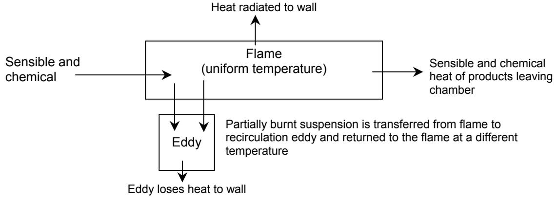
Fig. 4: Combustor sample for isothermal version
