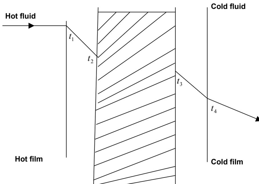
Fig.2: Temperature distribution for heat transfer across a metallic wall
